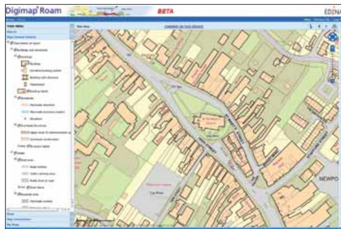
Roam Plan View - A large scale (view scale approx 1:1250) using OS MasterMap. The Map Content Control tab is show active. This presents a legend which can be used to customise the viewed map, by turning on or off map features, such as buildings, roads etc.
